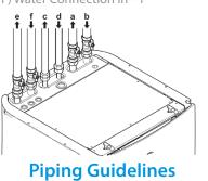
Minimum: 3m Maximum: Visit HSN Height Difference: 10m Min Flow Rate: 20L/min
