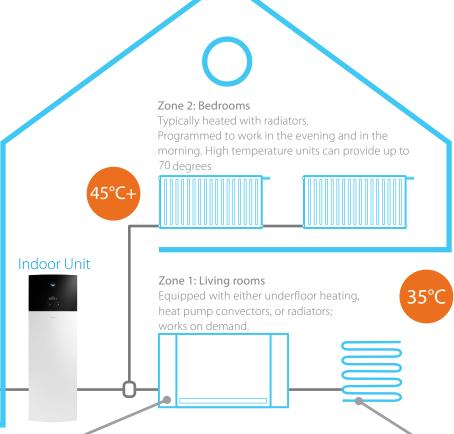
Fan coils, also called heat pump convectors, are hydronic emitters that can provide cooling or heating. A perfect addition to any home for cold winter nights or hot summer days
