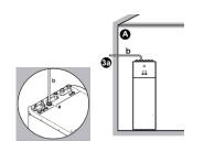
Chimney pipe to be routed externally based on R32 requirements
